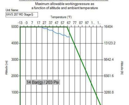
Graph represents working conditions, for starting conditions pls contact your Atlas Copco contact
